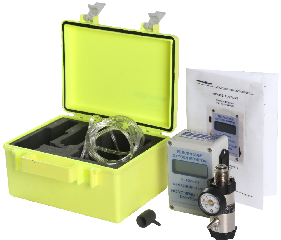
300 bar cylinder connector regulator to bleed off gas at low pressure for testing
