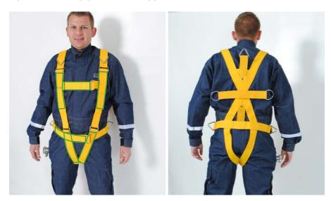
In order to don the harness: step into the leg holes, pull the harness over shoulders, tighten the straps (see highlighted green above) evenly at each adjustment point so that the harness is snug but comfortable.
