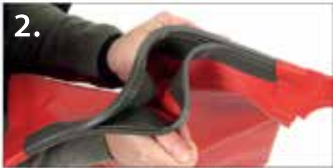
2. Squeeze and kink the seal into both hands and create an 'S' shape
